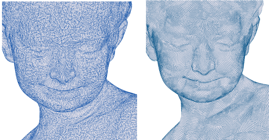
Figure 9: Principal direction estimation on Bimba (no noise). We put a line-segment aligned at every point to the minimal principal direction. Left: Jet-fitting method (with a polynomial of degree 4 \times 4 and k = 100 neighbors for each point). Right: d_{P,k}^w -VCM method (parameters R = 0.04 , r = 0.08 , k = 30 )
