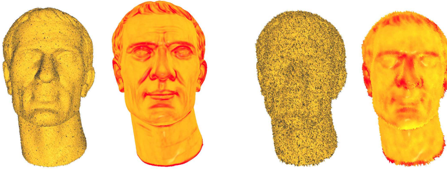
Figure 11: Mean absolute curvature on “ceasar” data estimated with d_{P,k}^w -VCM (yellow is low curvature while red is high curvature). Parameters are set as R = 0.04 , r = 0.04 , k = 30 . From left to right: input data with Hausdorff noise = 0.02; corresponding curvature estimation; input data with Hausdorff noise = 0.06; corresponding curvature estimation.
