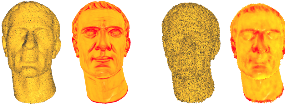
Figure 11: Mean absolute curvature on “cesar” data (of diameter D ) estimated with d_{P,k}^v -VCM (yellow is low curvature while red is high curvature). Parameters are set as R = 0.04D , r = 0.04D , k = 30 . From left to right: input data with Hausdorff noise = 0.02D ; corresponding curvature estimation; input data with Hausdorff noise = 0.06D ; corresponding curvature estimation.
