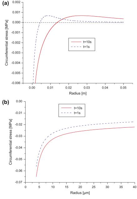
Fig. 5. The circumferential stress distribution at various times for a unit heat source  $q = 1 \text{ W m}^{-1}$  and  $r_R = 4 \mu\text{m}$ ; (a) general view, (b) enlargement near the reverse cyclic plastic zone.
