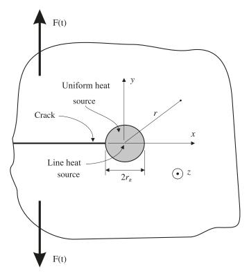
**Fig. 1.** Schematic of the thermomecanical problem of a semi-infinite crack in an infinite plate under cyclic tension (mode I) caused by a remotely mechanical loading F(t).
