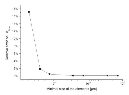
Fig. 8. Relative error on the stress intensity factor  $K_{l,temp}$  due to thermal stresses versus to the minimal element size for the finite element analysis.
