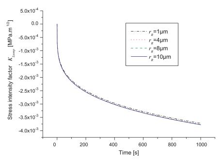
Fig. 7. The stress intensity factor  $K_{l,temp}$  due to thermal stresses versus time for different radius of the reverse cyclic plastic zone.
