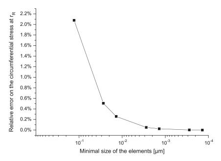
**Fig. 6.** Error on the circumferential stress  $\sigma_{\theta}$  at  $r = r_R$  versus the minimal element size for finite element simulation.
