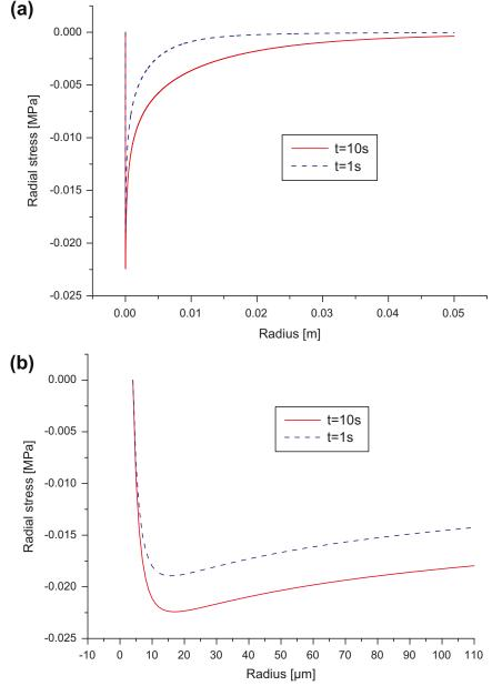
**Fig. 4.** The distribution of the radial normal stress for various times for a unit heat source  $q = 1 \text{ W m}^{-1}$  and  $r_R = 4 \mu\text{m}$ ; (a) general view, (b) enlargement near the reverse cyclic plastic zone.
