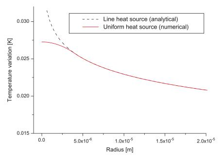
**Fig. 3.** Comparison of the temperature variation field for time t = 10 s in the case of a line heat source (analytic solution) and for a uniform radius heat source (numerical solution) both equal to 1 W m<sup>-1</sup>.
