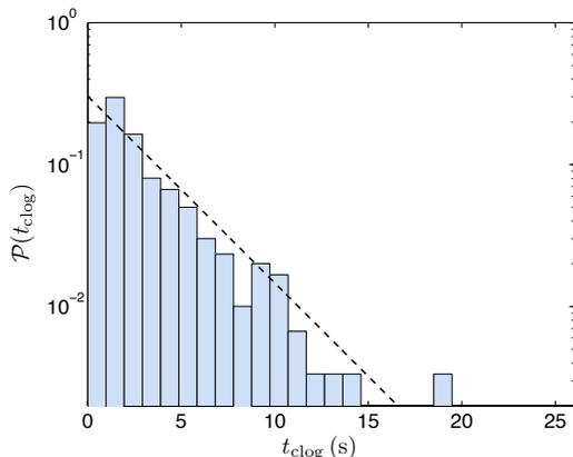
FIG. 3. Distribution of clogging time intervals  $t_{\text{clog}}$  for  $\Delta p = 13.8$  kPa and  $\phi = 2 \times 10^{-3}$ . The black dotted line is the best fit assuming a Poisson distribution with  $\langle t_{\text{clog}} \rangle = 3.3$  s.
