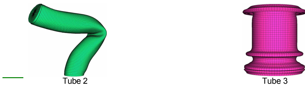
Fig. 11 Crushed shapes of the Tube 2 and the Tube 3 filled with a foam of 91.5 % of porosity, showing that progressive crushing mode changes from non-symmetric mode into Euler-type buckling mode and concertina mode for the Tube 2 and Tube 3, respectively
