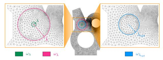
Figure 8. Definition of subdomains  $\omega_{\lambda}$ ,  $\omega_{\bar{\lambda}}$  involved in the first improved technique and  $\omega_{\bar{\lambda}_{\mathrm{opt}}}$  involved in the second one for quantity of interest  $I_1$ .
