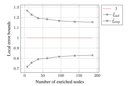
Figure 11. Evolutions of the lower and upper normalized bounds  $(\bar{\xi}_{\mathrm{inf}}, \bar{\xi}_{\mathrm{sup}})$  of  $I_{ex}$  for local quantity  $I_2$ , obtained using the classical bounding technique combined with handbook techniques, with respect to the number of enriched nodes.
