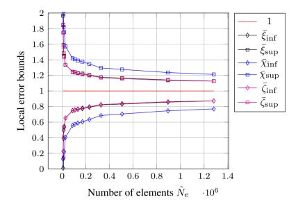
Figure 17. Evolutions of the lower and upper normalized bounds of  $I_{ex}$  for local quantity  $I_3$ , obtained using the classical bounding technique as well as first and second improvements, with respect to the number of elements  $\tilde{N}_e$  associated to the discretization of the adjoint problem.
