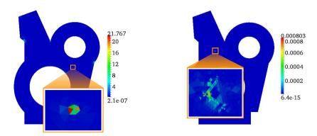
Figure 7. Spatial distribution of local contributions to the error estimates associated to reference (left) and adjoint (right) problems related to local quantity  $I_1$ . Zoom boxes represent the estimated errors in the vicinity of the crack tip for reference problem (left) and around the zone of interest for adjoint problem (right).
