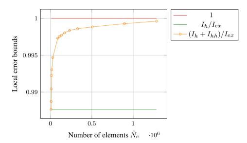
Figure 18. Evolutions of the normalized exact value of local quantity  $I_3$ , its normalized approximate value  $I_h/I_{ex}$  and its new normalized approximate value  $(I_h+I_{hh})/I_{ex}$  with respect to the number of elements  $\tilde{N}_e$  associated to the discretization of the adjoint problem.
