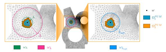
Figure 14. Definition of subdomains  $\omega_{\lambda}$ ,  $\omega_{\bar{\lambda}}$  involved in the first improved technique and  $\omega_{\bar{\lambda}_{\mathrm{opt}}}$  involved in the second one for quantity of interest  $I_2$  with two layers of nodes involved in the enrichment.
