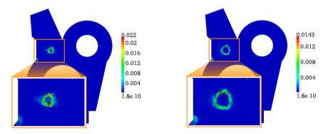
Figure 12. Spatial distribution of local contributions to the error estimates associated to (residual) adjoint problem related to local quantity  $I_2$ , with one (left) and two (right) layers of nodes involved in the enrichment. Zoom boxes represent the estimated errors around enriched zone  $\Omega^{PUM}$ .
