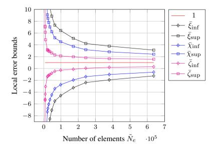
Figure 9. Evolutions of the lower and upper normalized bounds of  $I_{ex}$  for local quantity  $I_1$ , obtained using the classical bounding technique as well as first and second improvements, with respect to the number of elements  $\tilde{N}_e$  associated to the discretization of the adjoint problem.
