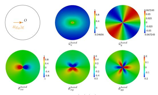
Figure 4. Spatial distribution of handbook pair  $(\underline{\tilde{u}}^{hand}, \tilde{\sigma}^{hand})$  associated to a pointwise force loading  $\delta(\underline{x}_O)\underline{x}$  applied to point O over an infinite domain,  $\underline{x}_O$  being the position of point O.
