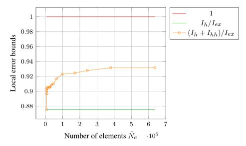
Figure 10. Evolutions of the normalized exact value of local quantity  $I_1$ , its normalized approximate value  $I_h/I_{ex}$  and its new normalized approximate value  $(I_h+I_{hh})/I_{ex}$  with respect to the number of elements  $\tilde{N}_e$  associated to the discretization of the adjoint problem.
