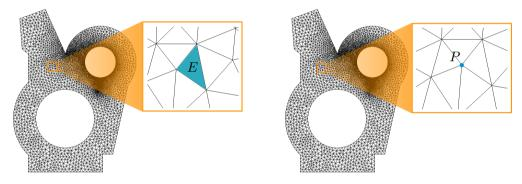
Figure 3. Position of element E (left) and point P (right) in the FE mesh defining the zones of interest for local quantities  $I_1$  and  $I_2$ , respectively.
