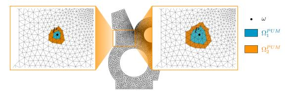
Figure 5. Definition of the zone of interest  $\omega$ , the subregions  $\Omega_1^{PUM}$  and  $\Omega_2^{PUM}$  in the enriched region  $\Omega^{PUM}$  for quantity of interest  $I_2$ ; enrichment with the PUM is applied to one layer (left) or two layers (right) of nodes.
