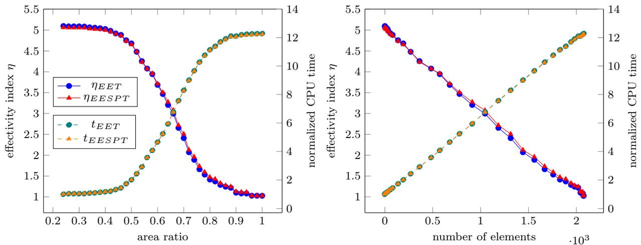
**Fig. 25** Effectivity indices and normalized CPU time for the error estimates EET and EESPT with respect to the area ratio (left) and to the number of elements involved in the optimized procedure (right).
