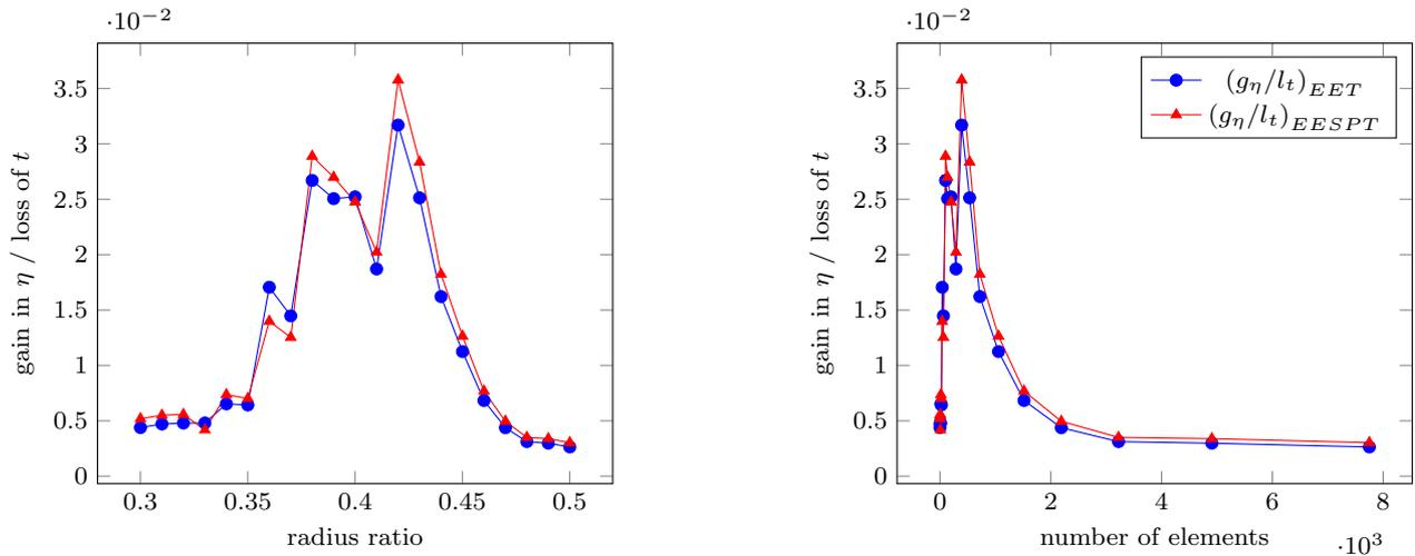
**Fig. 9** Ratio between gain in effectivity index and loss of normalized CPU time for the error estimates EET and EESPT with respect to the radius ratio (left) and to the number of elements involved in the optimized procedure (right).
