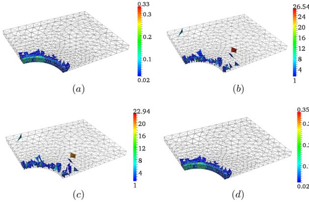
**Fig. 23** Spatial distribution of relevant local contributions to the density of the energy norm of the reference error (a) and that of the contributions to the density of the error estimates calculated using the standard versions of the EET (b) and the EESPT (c), and the full enhanced version (d).
