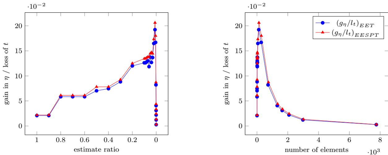
**Fig. 11** Ratio between gain in effectivity index and loss of normalized CPU time for the error estimates EET and EESPT with respect to the estimate ratio (left) and to the number of elements involved in the optimized procedure (right).
