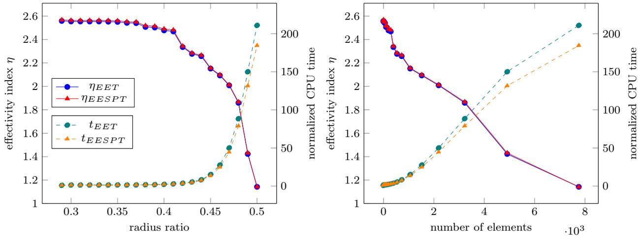
**Fig. 6** Effectivity indices and normalized CPU time for the error estimates EET and EESPT with respect to the radius ratio (left) and to the number of elements involved in the optimized procedure (right).
