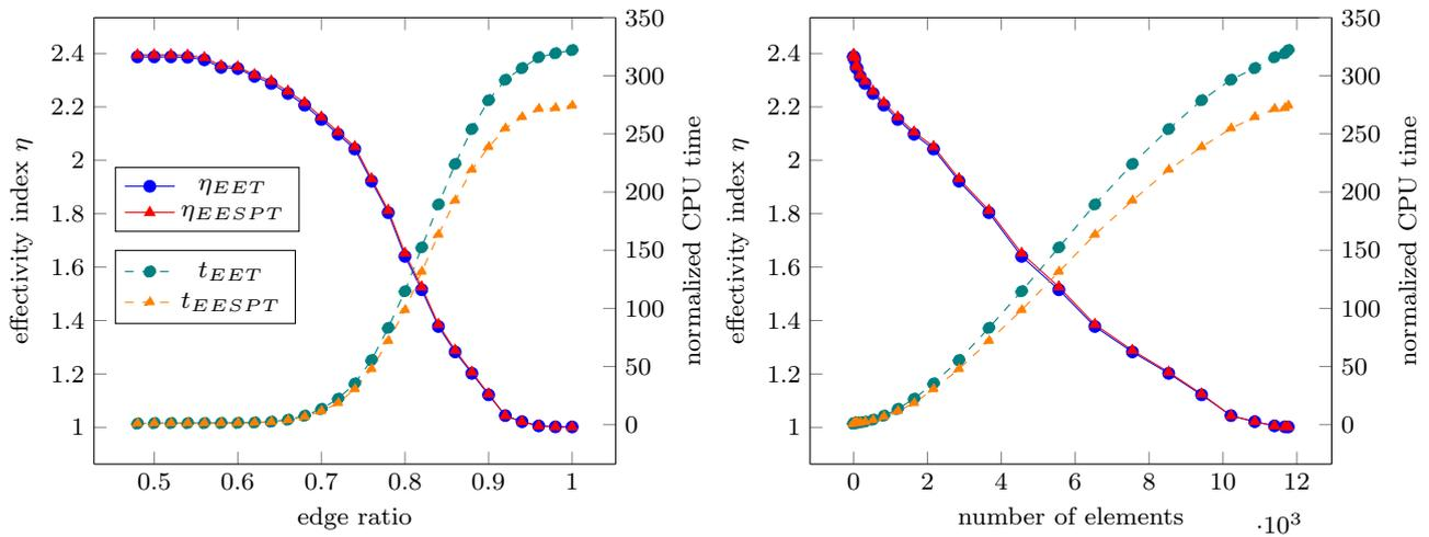
**Fig. 16** Effectivity indices and normalized CPU time for the error estimates EET and EESPT with respect to the edge ratio (left) and to the number of elements involved in the optimized procedure (right).
