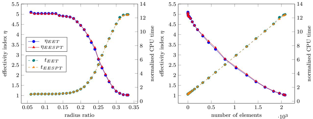
**Fig. 24** Effectivity indices and normalized CPU time for the error estimates EET and EESPT with respect to the radius ratio (left) and to the number of elements involved in the optimized procedure (right).
