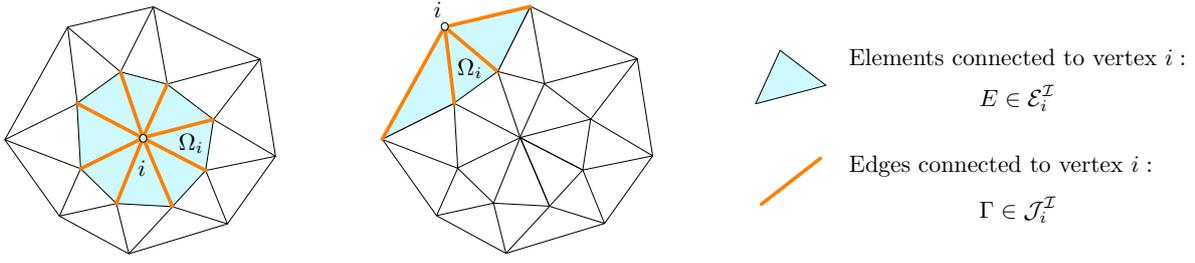
**Fig. 2** Elements and edges connected to vertex  $i$ .
