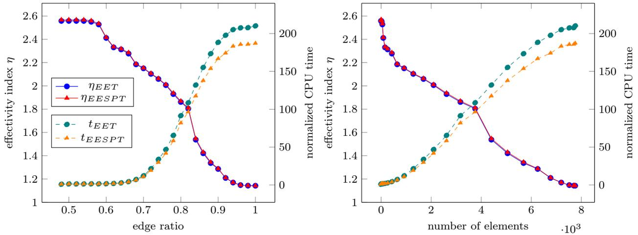
**Fig. 7** Effectivity indices and normalized CPU time for the error estimates EET and EESPT with respect to the edge ratio (left) and to the number of elements involved in the optimized procedure (right).
