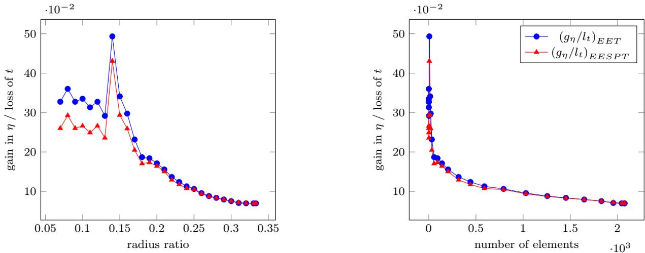
**Fig. 27** Ratio between gain in effectivity index and loss of normalized CPU time for the error estimates EET and EESPT with respect to the radius ratio (left) and to the number of elements involved in the optimized procedure (right).
