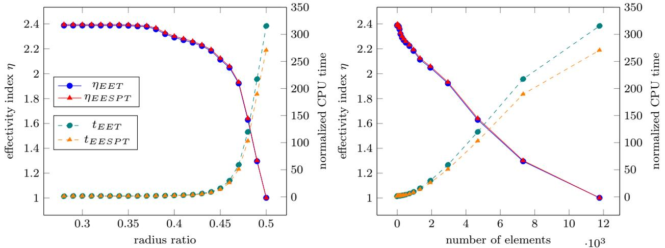
**Fig. 15** Effectivity indices and normalized CPU time for the error estimates EET and EESPT with respect to the radius ratio (left) and to the number of elements involved in the optimized procedure (right).
