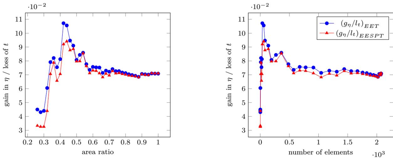
**Fig. 28** Ratio between gain in effectivity index and loss of normalized CPU time for the error estimates EET and EESPT with respect to the area ratio (left) and to the number of elements involved in the optimized procedure (right).
