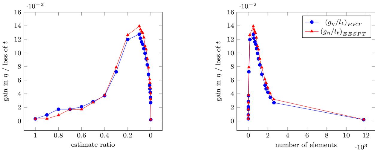
**Fig. 20** Ratio between gain in effectivity index and loss of normalized CPU time for the error estimates EET and EESPT with respect to the estimate ratio (left) and to the number of elements involved in the optimized procedure (right).
