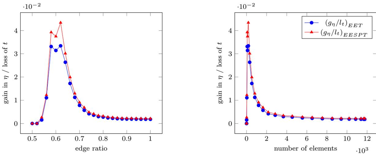
**Fig. 19** Ratio between gain in effectivity index and loss of normalized CPU time for the error estimates EET and EESPT with respect to the edge ratio (left) and to the number of elements involved in the optimized procedure (right).
