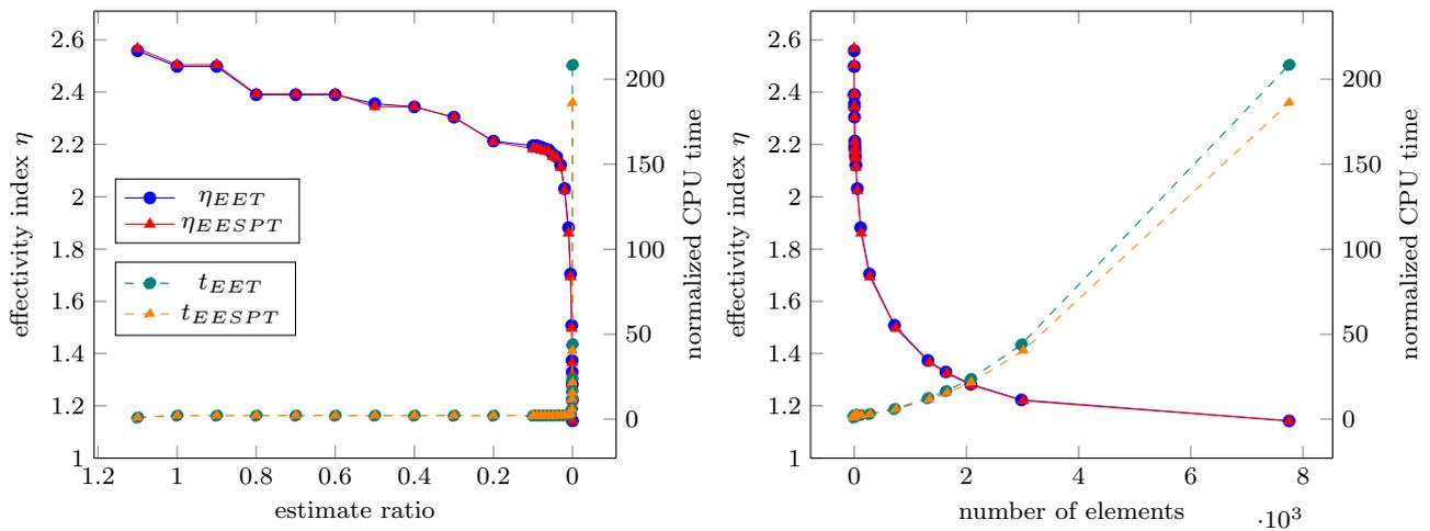
**Fig. 8** Effectivity indices and normalized CPU time for the error estimates EET and EESPT with respect to the estimate ratio (left) and to the number of elements involved in the optimized procedure (right).
