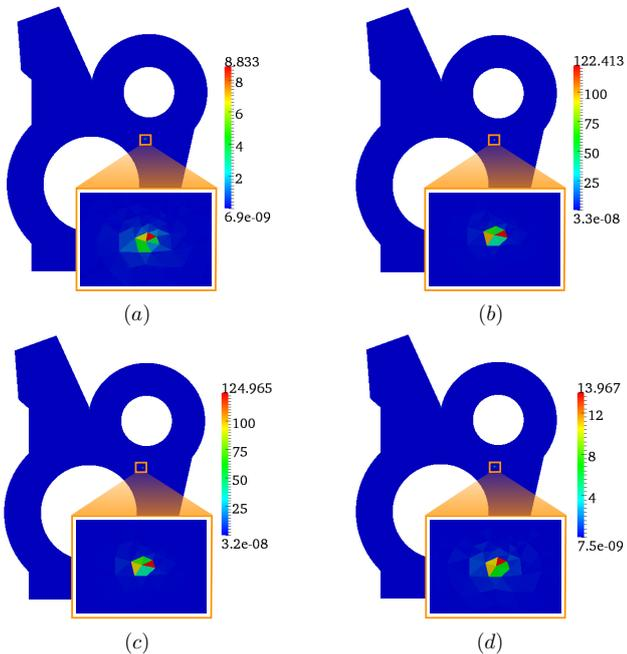
**Fig. 5** Spatial distribution of local contributions to the density of the energy norm of the reference error (a) and that of the contributions to the density of the error estimates calculated using the standard versions of the EET (b) and the EESPT (c), and the full enhanced version (d).
