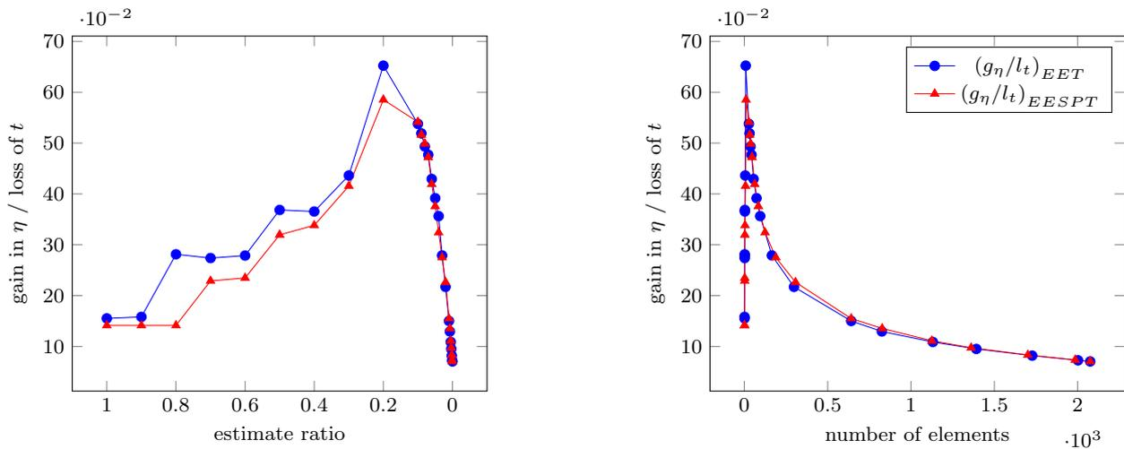
**Fig. 29** Ratio between gain in effectivity index and loss of normalized CPU time for the error estimates EET and EESPT with respect to the estimate ratio (left) and to the number of elements involved in the optimized procedure (right).
