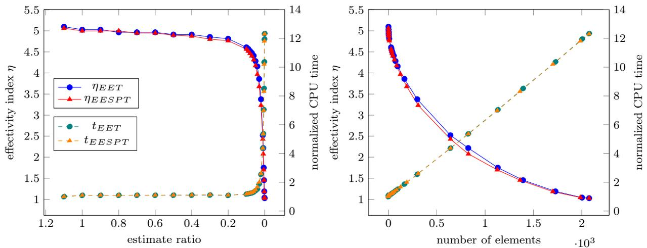
**Fig. 26** Effectivity indices and normalized CPU time for the error estimates EET and EESPT with respect to the estimate ratio (left) and to the number of elements involved in the optimized procedure (right).
