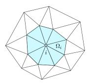
Figure 2. Patch  $\Omega_i$  associated with vertex i.
