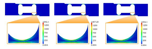
Figure 7. Magnitude of the admissible stress field calculated using the EET (left), the SPET (center), and the EESPT (right). Zoom boxes represent the admissible stress fields in the vicinity of the bottom region of the right hole.
