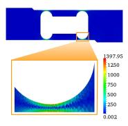
Figure 6. Magnitude of the FE stress field and zoom around the highly-loaded region.
