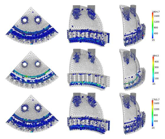
Figure 22. Spatial distribution of relevant local contributions to the density of the error estimates calculated using the EET (top), the SPET (middle), and the EESPT (bottom).
