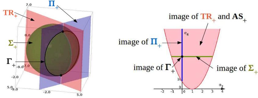
Figure 3: Left: picture of  $\text{AS}_+$ , 3-d component of actuation singularities in the workspace. Right: Picture of  $\mathbf{P}_+$ , plane in the joint space containing the image of  $\text{AS}_+$  under IKM
