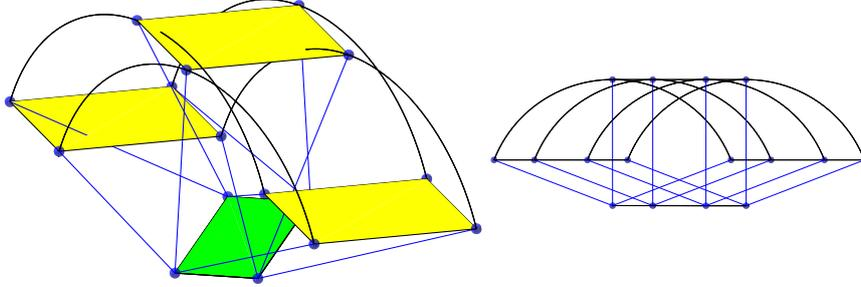
Figure 4: Two viewpoints on self-motion along vertical circle in the Schoenflies mode. The top pose is a transition to an extra mode of operation
