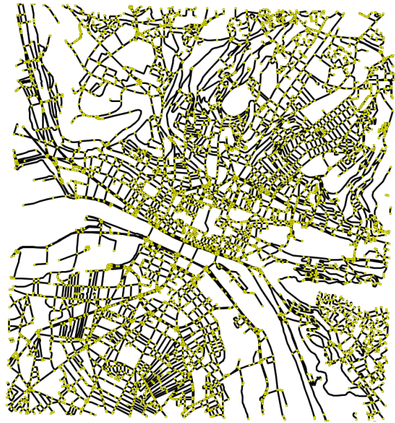
Figure 7: Total area simulated: in black the roads and in yellow the nodes
