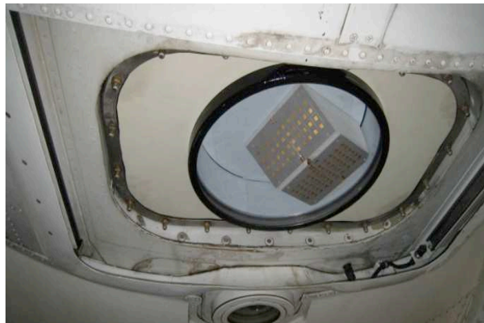
Figure 6. External view of both antennae aiming through the quartz windows
