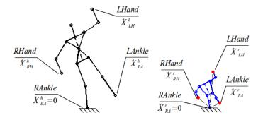
**Fig. 1.** Scaling process from human body (left) to humanoid robot (right). Step 1: human to humanoid joint positions (blue); Step 2: end-effectors positions (red).
