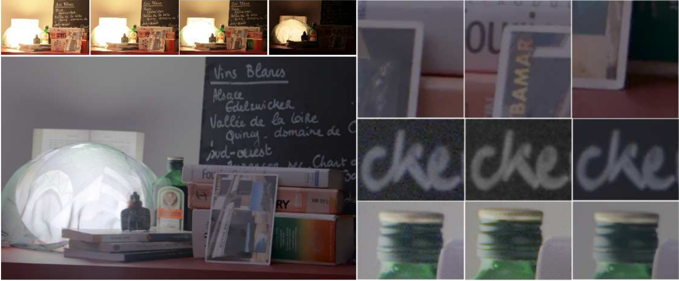
Figure 5: Real data. Static scene except for one moving object (the postcard) acquired using a hand-held camera. Left side. First row: Input images (JPEG version). Second row: Tone mapped irradiance estimation using the proposed non local estimation approach. Right side. First row: Extracts of the moving object (the postcard). No ghosting artifacts appear. Second / Third row: Extracts of the normalized reference image (left), the method by Sen et al. [26] (center) and the proposed non local approach (right). The irradiance estimation of the proposed approach is considerably less noisy than the one obtained using the reference frame only or the method by Sen et al. Please see the electronic copy for better color and details reproduction.
