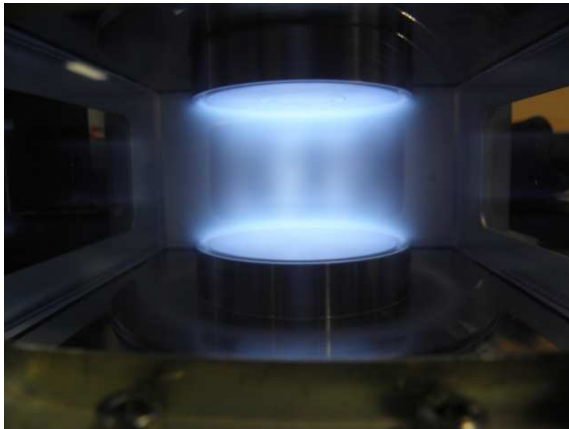
Fig. 1: Instabilities appearing during dust particle growth in a capacitively coupled rf discharge shown with a standard 24 fps CCD camera. They appear as striations in the emission of the Kr plasma.
