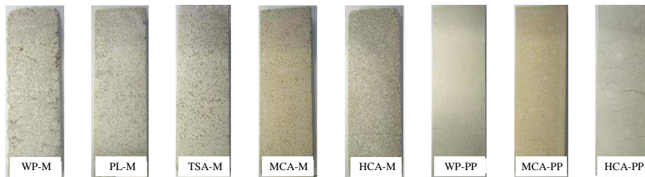
Fig. 4: Samples inoculated with Aspergillus niger after 72 days of incubation.
