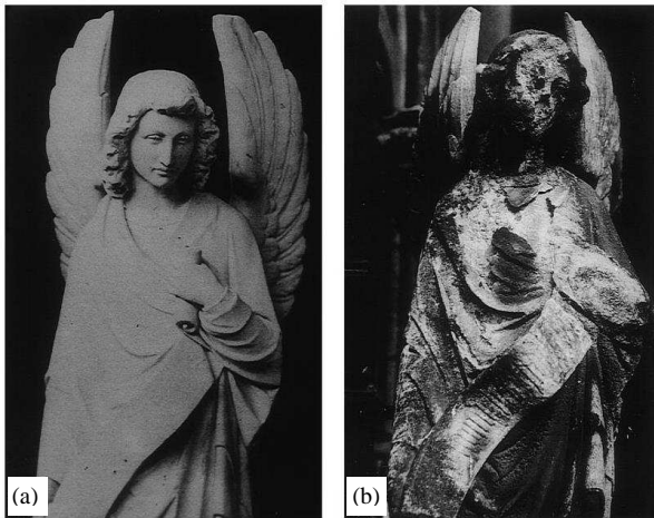
Fig. 1: Influence of biodeterioration process on an angel statue of the cathedral of Cologne (Germany), (a) original object in 1880 (photograph by Anselm Schmitz, Cologne) and (b) the respective weathered statue in 1993 (photograph by A. Wolff, Cologne)
