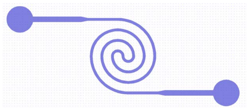
Fig. 5. Design of metal resistor Width: 20μm and Length: 4.62mm
