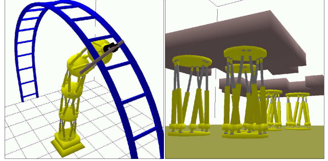
Fig. 8. Examples of associations of Stewart platforms.
