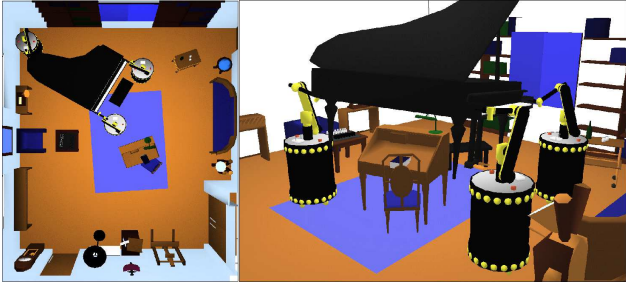
Fig. 10. A piano mover problem with three cooperating mobile arms.
