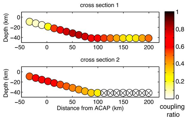
**Figure 8.** Cross-section of the coupling on the interface, along the two lines shown in Figure 7. Cross-section 1 is located in the Guerrero gap, similar to the cross-sections in Figure 6, and cross-section 2 is located below the ZIHP station, west of the Guerrero gap. The crossed white dots represent subfaults with insufficient resolution (restitution index  $< 0.85$ , Figure S6).
