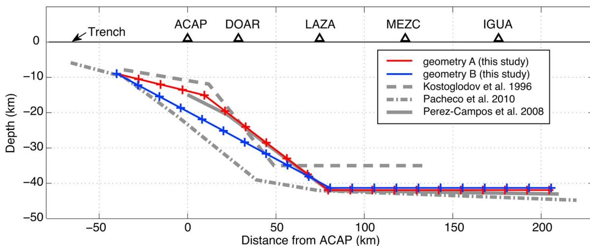
**Figure 3.** Geometries of the fault planes used in the present study, along a profile perpendicular to the trench (profile located below the line of inland GPS stations, from Acapulco (ACAP) to Mexico city). Red curves, geometry A; blue curve; geometry B; gray curves, principal geometries proposed in recent studies. Black triangles, GPS stations located on the profile. The distance from the GPS site ACAP to the Middle American Trench is 66 km. Vertical exaggeration by a factor of 2.
