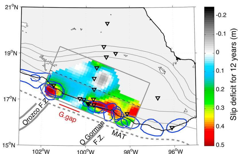
**Figure 9.** Slip deficit over 12 yr (geometry B). Slip contours of the major earthquakes are in blue. The slip deficit in the Guerrero gap is in average 1/4 of the slip deficit on both sides of the gap. Black triangles, GPS station locations. Thick dashed gray line, Middle American Trench (MAT). Thick continuous gray lines, fracture zones. The location of the northwest Guerrero gap (G.Gap) is shown in red.
