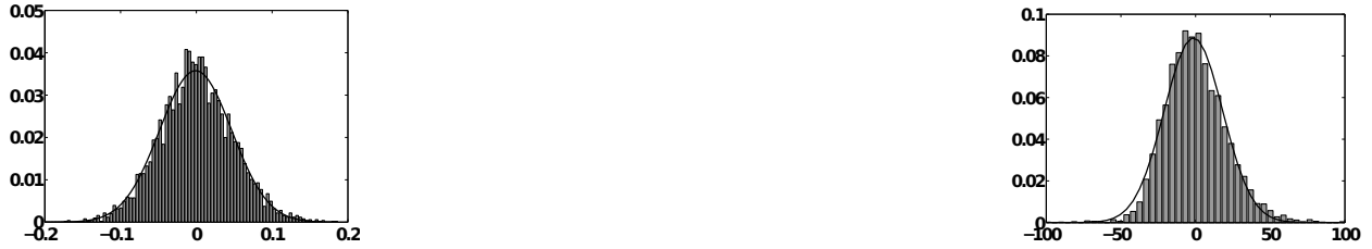
Fig. 9. Bars: Estimated probability density functions of the centered processes {}^c\tilde{A} (Left) and {}^c\tilde{\Delta}_T (Right). Solid line: Gaussian fit. For the sake of figure readability, the results are only displayed for the parameter set \kappa=5\cdot 10^9 \text{ N.m}^{-\alpha}.\text{kg}^{-1} , \mu=1 \text{ s.m}^{-1} and \beta=-0.5 . Readers can find figures for the others parameter sets on the accompanying website.
