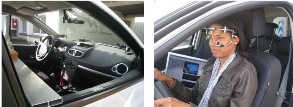
Fig. 3: Views of the CEREMA's instrumented vehicle (and instrumented driver).
