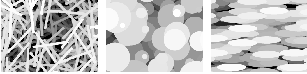
Figure 4: Realizations of three different Boolean random fields with uniformly distributed gray-levels. The grain distributions are the ones presented in Fig. 1.
