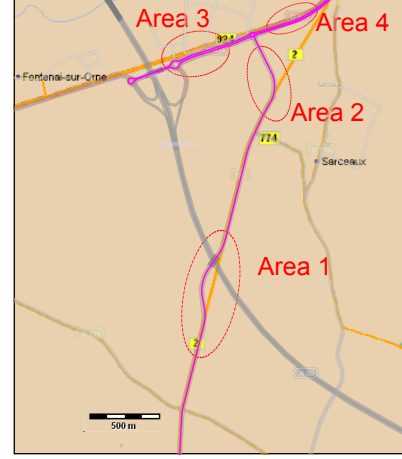
Fig. 4. Global top view of the test areas. The out-of-date map being assessed is shown by yellow lines. A map of the actual road network is plotted in transparent grey. The four test zones are circled in red. The trajectory followed by the vehicle is in purple.
