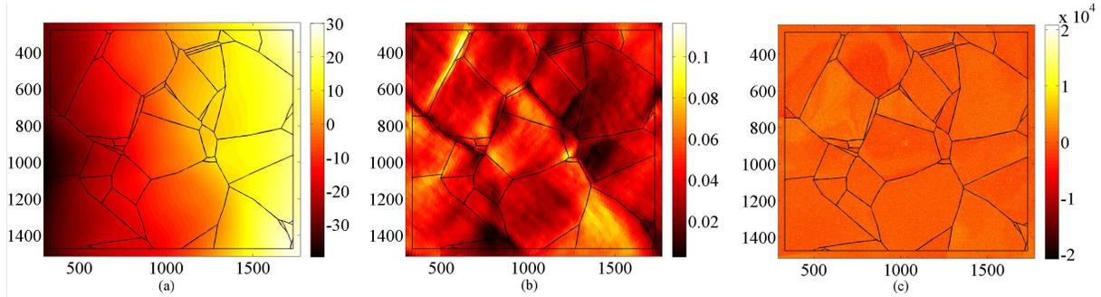
**Figure 2:** Displacement field expressed in pixels (a) and strain field (b) along the horizontal direction, measured experimentally for a macroscopic strain of 5%. The physical size of one pixel is 150 nm. Corresponding correlation residuals expressed in gray levels (c). The dynamic range of pictures is 16 bits. The grain boundaries are shown as black lines on these three fields
