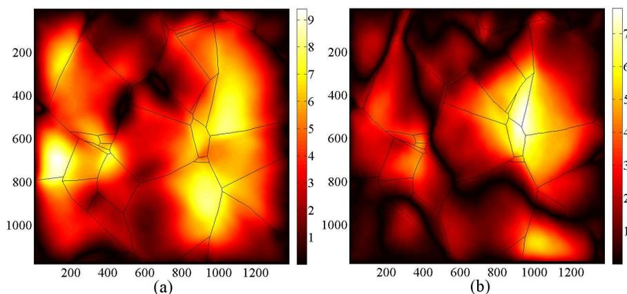
**Figure 3:** Absolute value of the difference between displacements fields expressed in pixels along the horizontal (a) and vertical (b) when measured by DIC and simulated by finite element computations for a macroscopic strain of 5 %. The set of parameters used for the simulation is that identified by homogenization. The physical size of one pixel is 150 nm. The grain boundaries are shown as black lines on these three fields.
