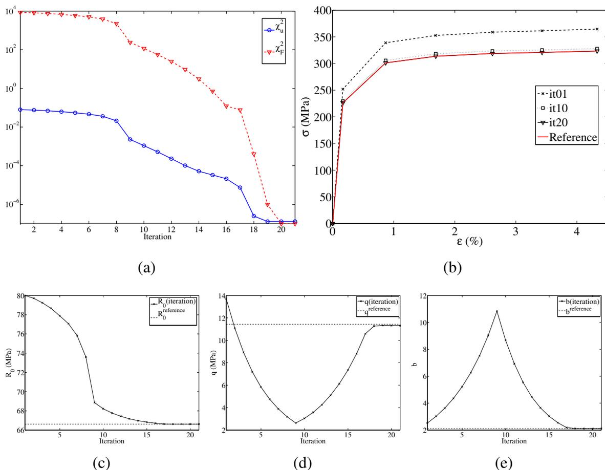
**Figure 4:** Numerical test case in which a set of reference values of the parameters is to be identified. Cost functions  $\chi_u$  and  $\chi_F$  as functions of the iteration of the identification procedure (a). Change of the macroscopic stress-strain curve wrt. iterations (b). Change of the parameters  $R_0$  (c),  $q$  (d) and  $b$  (e), as functions of the iteration
