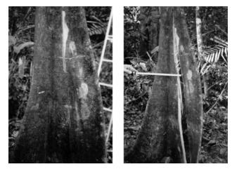
Fig. 7. Breakage observed during bending tests on the second *Sloanea* tree. The cracking buttress is lined up with the force direction and put in compression. Left, just after hearing the first crack; right, after increasing the load.
