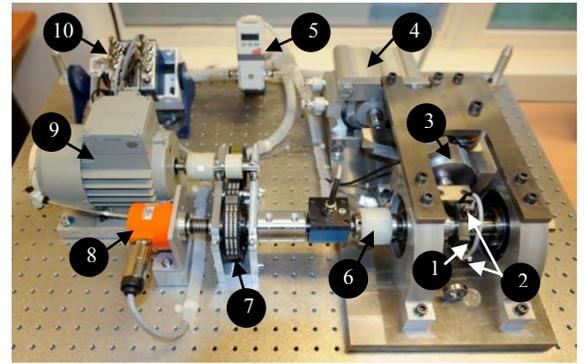
1- Test bearing    2-Accelerometers    3-Force sensor
