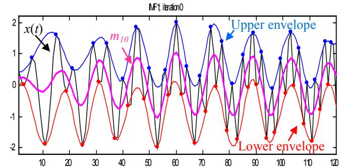
Fig. 2. Sifting process: original signal  $x(t)$  with the upper envelope (blue line) and lower (red line) and the resultant mean line  $m_{10}$  (purple line).
