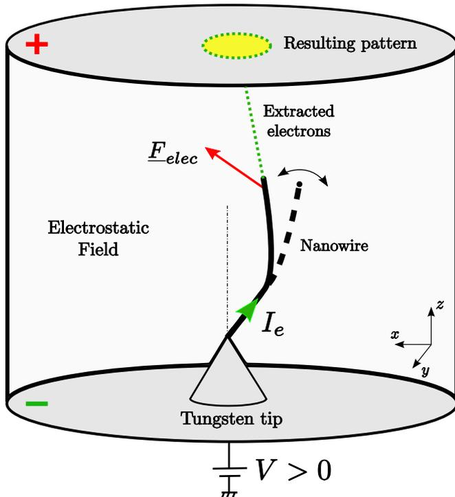
Fig. 1. Experimental settings: nanowire in field emission.
