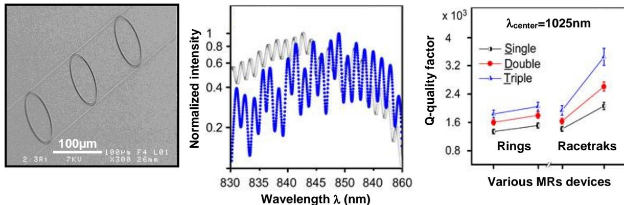
Fig. 2. SEM image of a cascade made of three ring micro-resonators (triple-cascade-MRs); resonances transmissions spectra at  $\lambda_{center}=845nm$  corresponding to a single-ring-MR and a cascade of triple-ring-MRs; evolution of the quality Q-factor values at  $\lambda_{center}=1025nm$  as a function of various family-MRs and configurations (single, double and triple MRs with ring and racetrack shapes with sundry geometrical dimensions).
