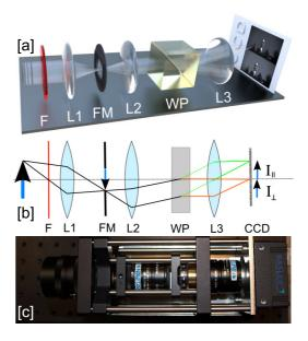
Fig. 2. Polarimetric imaging setup: The Wollaston prism (WP) angularly separates the incident beam into two orthogonal polarization components forming two images  $I_{\parallel}$  and  $I_{\perp}$  on the CCD. The illustration in (a) shows a orthographic view of the polarimetric imager while the schematic in (b) geometrically indicates the working principle of the imaging setup. A top view photograph of the imaging setup is shown in (c).
