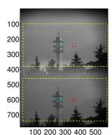
Fig. 4. The raw image obtained from the camera with  $782 \times 582$  pixels. Extraction of two image channels after applying image registration process is demarcated in yellow dashed box. The ambient illumination is obtained by averaging over the region shown in red-dashed lines and the region shown in blue dashed lines is the  $21 \times 21$  pixels ROI that includes the source at its center.
