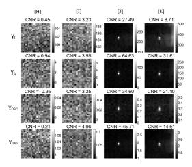
Fig. 6. CNR images of the 21  $\times$  21 region of interest around the polarized light source, extracted at times indicated by H, I, J and K in Fig. 5. Row 1 to 4 correspond to the CNR obtained with intensity image, difference image, OSC image and contrast ratio image respectively. The corresponding CNR for the central source pixel are also given as numerical figures for comparison.
