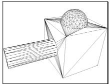
Figure 13: Simplification of a polyhedron with a small dimension of error zone. The vertices on the spherical surface have not been simplified but the vertices lying on cylindrical or plane surfaces have all been simplified.
