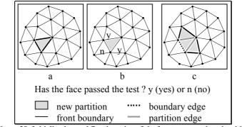
Figure 28: Initialization and first iteration of the front propagation algorithm
