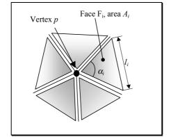
Figure 3: Geometric parameters of a star-set associated to a vertex *p*.
