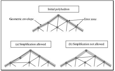
Figure 12: Principle of the simplification algorithm, the simplified polyhedron does not intersect each of the error zones (b) whereas it does (a)
