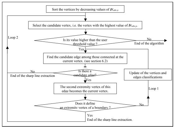
Figure 22: "Sharp lines" identification algorithm.
