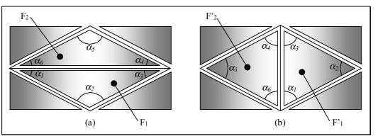
Figure 16: Parameters used by the  $F_e$  cost function before (a) and after (b) the edge swapping.
