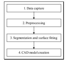
Figure 1: The main phases of a reverse engineering process.
