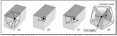
Figure 10: (a,b,c) the same geometry at vertex p is described by equivalent meshes, (d) circular sectors associated to the star-set of the vertex p.
