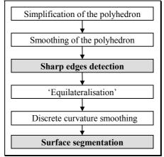
Figure 2: The main phases of the segmentation approach.
