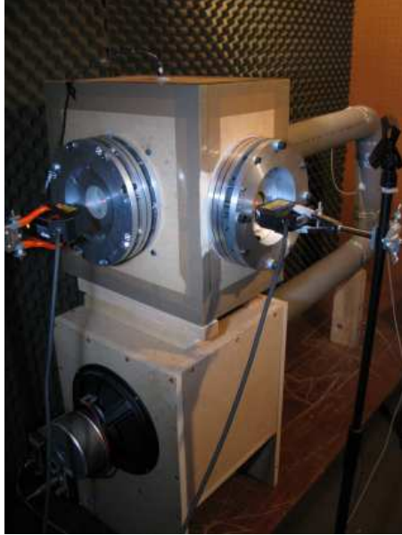
Figure 1: Experimental set-up with two membrane absorbers.
