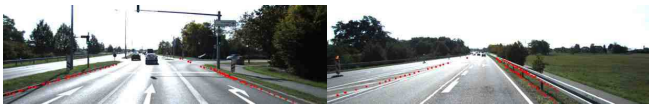
Figure 5: Projection of selected candidates into the RGB image. The right figure shows an example case where ground plane classification fails.
