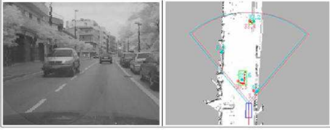
Fig. 4. Moving object detected from laser data is confirmed by radar data.
