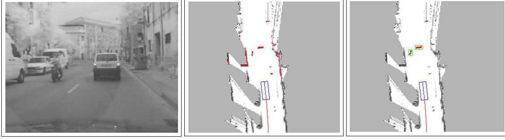
Fig. 7. Moving object detection example. See text for more details.
