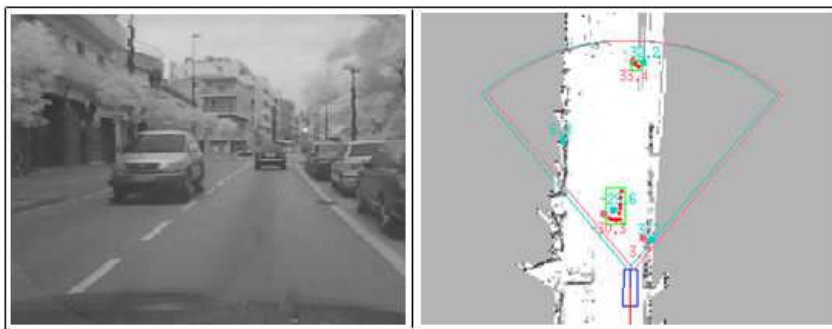
Fig. 8. Moving objects detected from laser data are confirmed by radar data.
