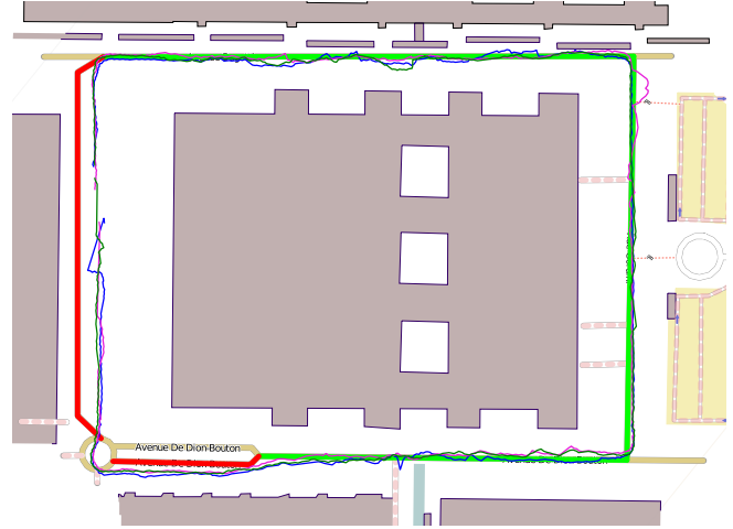
Fig. 6: Results of FDI in a urban environment after three journeys. The red links correspond to map errors that have been fully isolated during the third journey.
