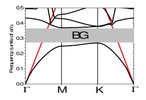
Figure 2 : band diagram of the triangular 2D-PhC membrane for a thickness T= 0.31 *a* and a 40% filling factor
