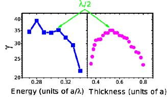
Figure 4 : SE enhancement factor as a function of energy (blue square, left) for thickness of 0.6 a, and as a
