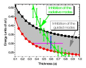
Figure 3 : Valence band edge (red round), conduction band edge (Black Square) of the 2D-PhC and frequency corresponding to a  $\lambda/2n$  thickness (green triangle), as a function of the membrane thickness
