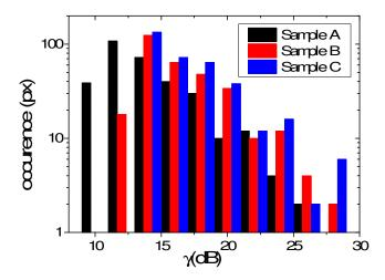
Figure 8 : Histogram of the occurrence of the calculated 10log(γ) on maps for the 3 structures, without Bragg mirror in black suspended on one Bragg mirror in red and sandwiched between 2 mirrors in blue.
