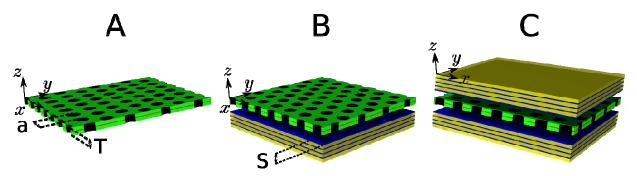
Figure 1 : Schemes of the studied structure, A- triangular 2D-Phc membrane suspended in air, B- triangular 2D-Phc suspended on the top of a Bragg mirror, C- triangular 2D-PhC sandwiched between two Bragg mirrors.
