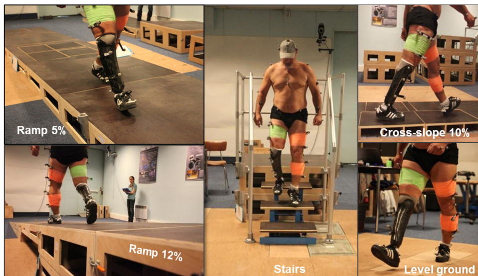
Fig. 1. Four reproduced situations in the gait laboratory.
