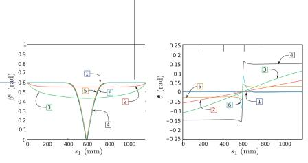
Fig. 6. Opening angle b°ds<sub>1</sub>p and rotation hds<sub>1</sub>p of the cross-section along the rod for the six deformed shapes shown in Fig. 5.
