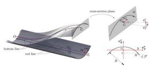
Fig. 2. Geometric and kinematic description of the tape spring (left) and its cross-section (right), with  $\delta O(e_1; e_2; e_3)$  the fixed orthonormal frame and  ${}^{\hat{y}}G(e_i^r) e_2^r$  of the rotated frame that follows the cross-section plane.
