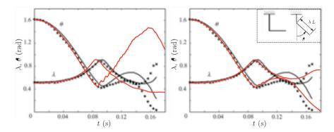
Fig. 13. Results obtained for test (a). Evolution of the fold angle h and the non-dimensionalized length k of the free straight part of the spring with respect to time. Crosses 1 and circles
