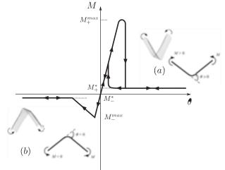
Fig. 4. Schematic response of a tape spring submitted to opposite rotations at ends: bending moment vs prescribed rotation (according to Seffen and Pellegrino (1999)), in opposite-sense bending (a) and equal-sense bending (b).
