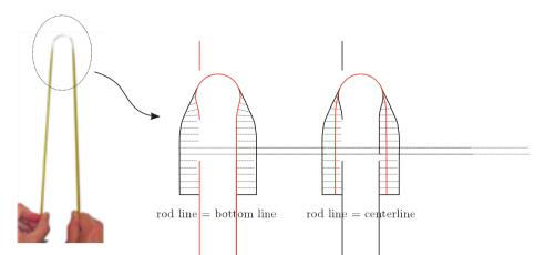
Fig. 3. Schematic folding of a tape spring with two straight and undeformed parts, a circular zone where the cross section is completely flattened, and two transition zones. The cross section planes are represented in dashed black lines and the rod lines are in red solid lines. In the transition zones the two choices for the reference line (bottom line or centerline) do not lead to the same kinematics when the orthogonality of the cross-section plane with respect to the rod line is considered.
