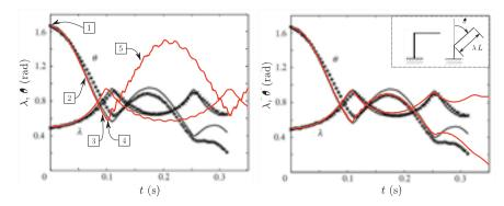
Fig. 11. Results obtained for test (b). Evolution of the fold angle h and the non-dimensionalized length k of the free straight part of the spring with respect to time. Crosses 1 and circles
