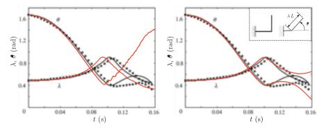
Fig. 14. Results obtained for test (c). Evolution of the fold angle h and the non-dimensionalized length k of the free straight part of the spring with respect to time. Crosses 1 and circles
