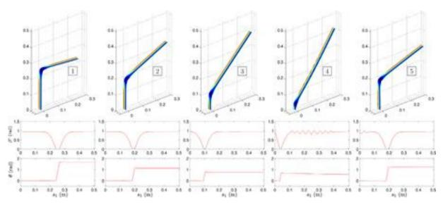
Fig. 12. Reconstructed deformed shapes of the tape at five significant time values during the deployment step for test (b), with superimposed color plots of angle b. From 1 to 5: t=0, 0.06, 0.085, 0.102 and 0.16 s. Bottom plots: opening angle  $b^{\dagger}\delta_{s1}^{\dagger}$  and rotation  $h\delta_{s1}^{\dagger}$  of the cross-section plane along the rod for the five deformed shapes.
