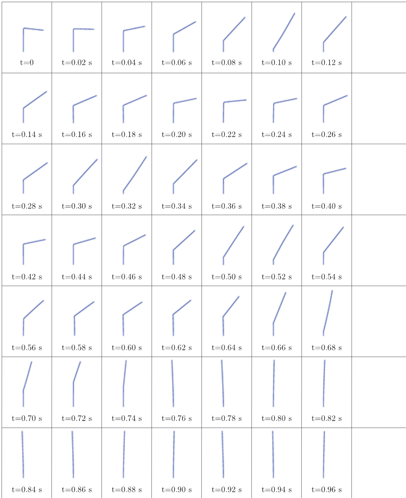
Fig. 10. Deformed shape of the rod line during the deployment step for test (b). It shows the traveling of the fold along the tape spring between the middle and the bottom of the tape with a rebound phenomenon at the bottom. The fold disappears after the fourth rebound and the tape then behaves as a beam which oscillates according to the first free-vibration bending mode.
