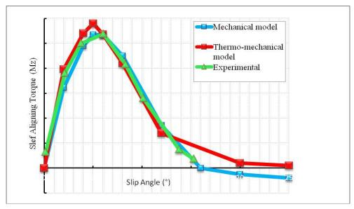
Fig.6. Comparison between experimental data, mechanical and thermo-mechanical models Self aligning torque  $M_{\rm z},\,$
