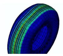
Fig.8. Temperature gradient for a cornering simulation at given velocity and slip angle
