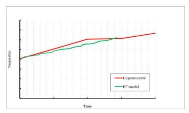
Fig.9. Temperature evolution: comparison between thermomechanical FEM and Experimental data for a cornering simulation of an aircraft tyre for given velocity and slip angle
