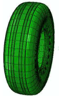
Fig.2.3-D fully coupled thermo-mechanical model
