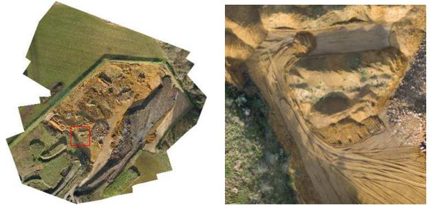
Figure 4. Orthoimage of the  $450 \times 450m^2$  mapped area (the right inset is a zoomed view of the red square in the left image).
