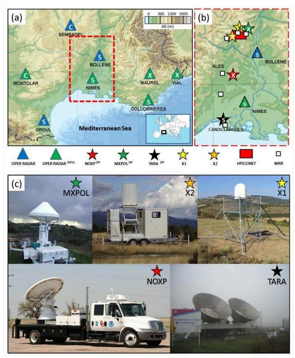
**Figure 1:** Overview of the HyMeX radar network in Southern France during SOP1. (a) Operational radars, (b) Research radars deployed in the Cevennes-Vivarais area (dashed red box in a), (c) Pictures of the main research radars. Color shadings in (a-b) show terrain height. Symbol DP indicates dual-polarization systems. Symbols S, C and X indicate the radar wavelength.
