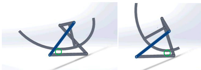
Figure 1. Model illustrating relationship between condyle radii and ligament lengths: (left) knee in extended position, (right) knee in flexed orientation. Note the gap between femur and tibia (green circles) is constant in this model, indicating compatibility between ligament and joint surfaces.
