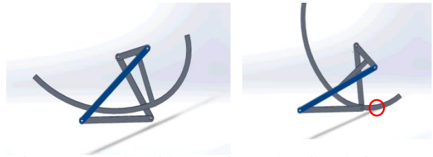
Figure 2. Model with same femoral radii as before, but sub-optimal ligament placement. In flexion, the femur is compressed into the tibia (red circle).
