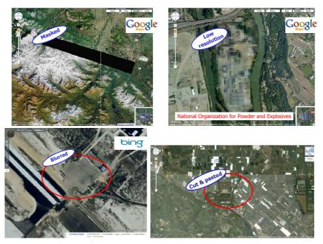
Fig. 1. Sensitive spatial objects protected with various methods
