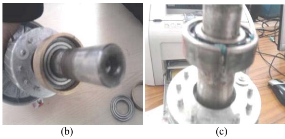
Figs. 2. Experimental set-up of 1.1 kW to collect healthy and faulty induction machine data in stator current
