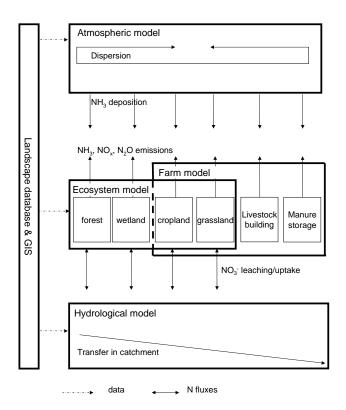
Fig. 1. The NitroScape model scheme.
