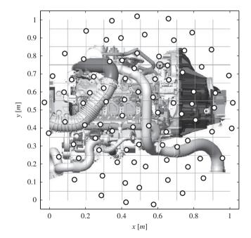
Fig. 7. Scheme of the 84-microphone irregular array with uniform density used for the MAH measurements. Each spot corresponds to a microphone position.
