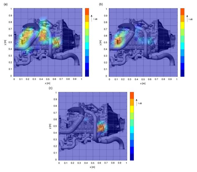
**Fig. 8.** Separation of the overall sound intensity radiated by the top side of a 1998cc diesel engine into a contribution from the combustion source and a contribution from the injection noise. The engine speed is 800 rev/min and the active sound intensity is displayed in the 1250 Hz 1/3-octave band. (a) Overall sound intensity, (b) contribution of the combustion source, (c) contribution of the injection noise.
