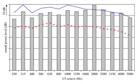
Fig. 6. Sound power emitted by an exhaust face engine operating at 3000 rev/min at full charge. Bar chart: overall level; solid line: power contribution from combustion sources returned by a commercial solution; dotted line: power contribution from combustion source returned by the cyclic Wiener filter.
