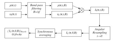
Fig. 3. Computation process of the cyclic sound intensity.
