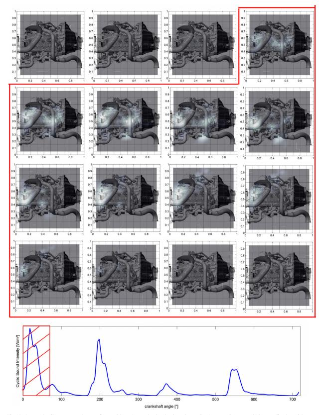
**Fig. 10.** Consecutive frames composing a cyclic sound intensity movie, showing how the combustion part of the acoustical energy flux is evolving as a function of the crankshaft angle ( $\Delta\theta$  = 3.7<sup>-</sup>) on the top side of a diesel engine operating at 800 rev/min, in the 1250 Hz 1/3-octave band. The frames correspond to the hatched area of the cyclic sound intensity on the engine top side displayed in the bottom panel.
