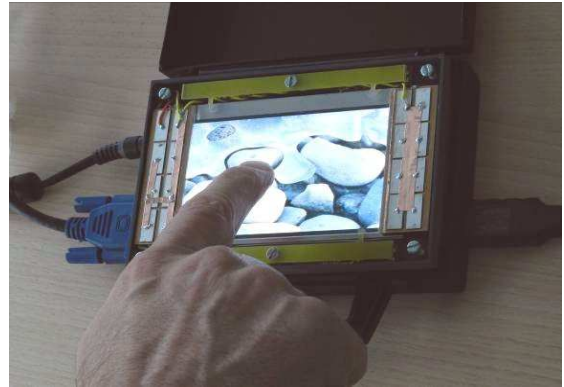
Figure 6. The transparent prototype with its exciters
