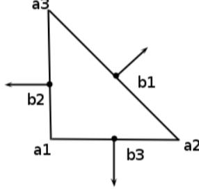
FIG. 3. The quadratic Morley finite element geometry
